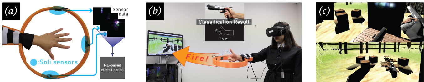
Figure 1: The VRTwitch setup; a) VRTwitch controller has three Soli sensors mounted on a 3D-printed housing, b) a player performs a micro gesture to manipulate a gun in the VR experience, c) screen captures of the demo experience
