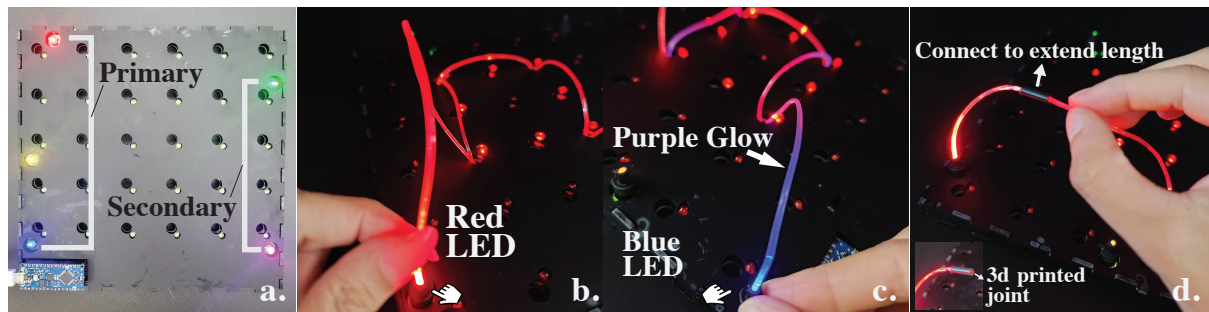
Fig. 5. TIEboard color theory: (a) 3 Primary colors from color wheel (RYB) and 2 secondary colors (b) Insert end of fiber in red LED (c) Mix red and blue color: Insert other end in blue and produce purple color (d) 3D printed part to extend the length of string
