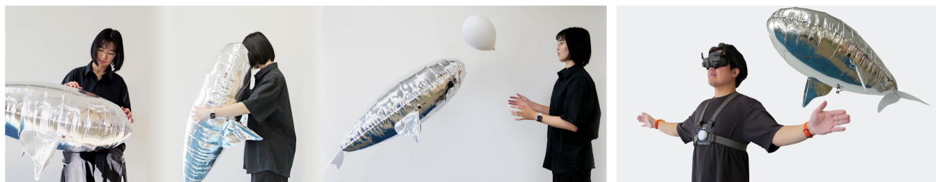
Figure 1: The concept of using the soft floating robotic avatar for physical interaction: A pilot wearing a body-tracking interface embodies a fish-shaped avatar, "swimming" through the remote environment to engage with others in physical interactions.
