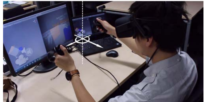
Figure 1. PinchMove being used bimanually, where the user's translation and axis of rotation are about the hands to achieve accurate navigation virtually.
