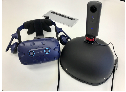
Figure 2: Our prototype consists of HTC Vive Pro Eye and Ricoh Theta V mounted on helmet.
