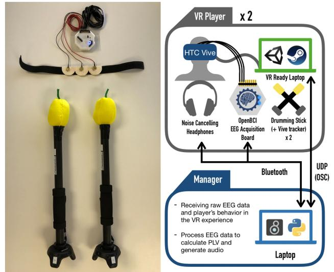
Figure 2: EEG headband and drum sticks used (left) with the system overview (right)
