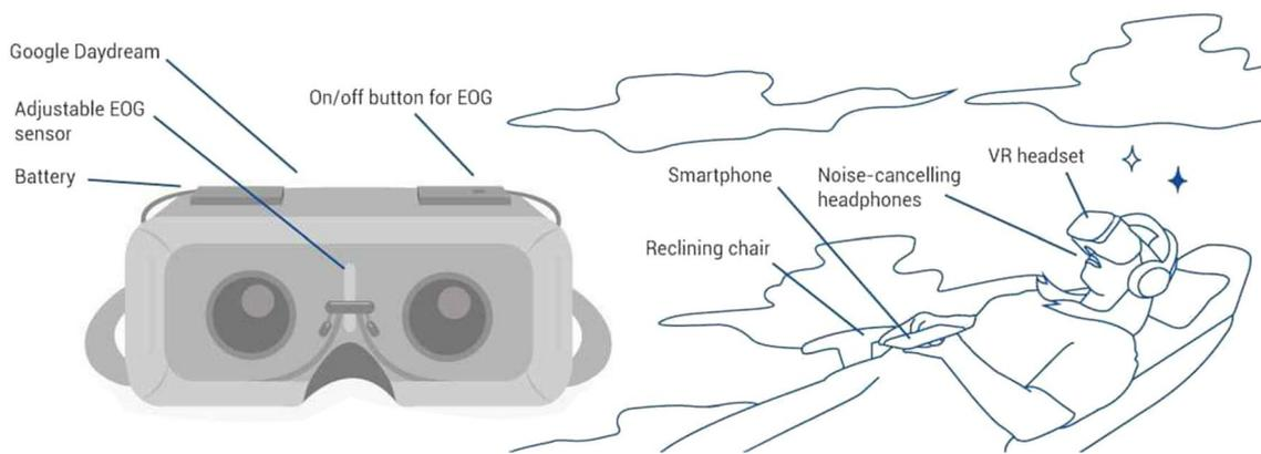
**Fig. 1** (left) An illustration of the prototype that combines EOG sensors from JINS Meme with Google Daydream, (right) and a participant of the study using the prototype on a reclining office chair with a smartphone for a finger tapping task to detect sleep onset manually
