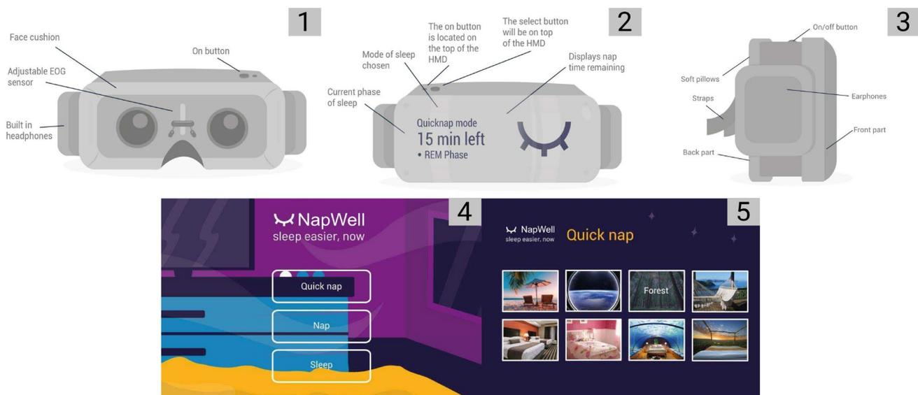
**Fig. 9** Envisioned prototype with (1) adjustable EOG sensors and face cushion, (2) an outward display showing the sleep mode and remaining period, (3) integrated headphones, (4) the home screen
