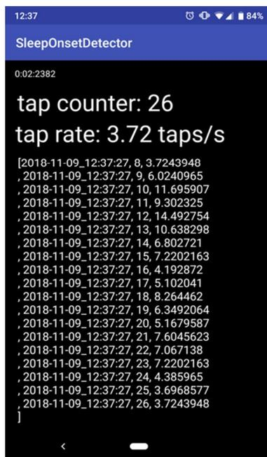
**Fig. 2** Screen capture of the FTT application logging the time stamp, tap number, and tap rate
