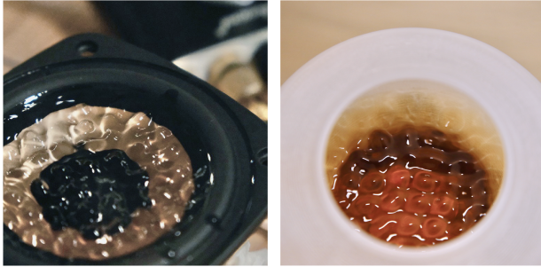
Figure 11: The comparison between an exposed speaker and Cymatics Cup
