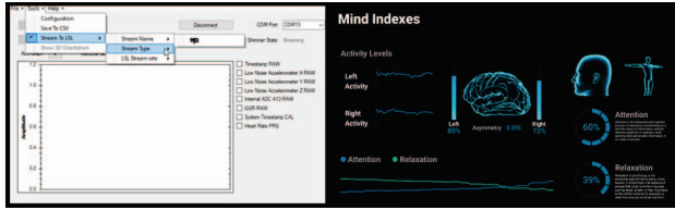
Fig. 4. We created a standalone application to collect data from the shimmer3 sensor via Bluetooth and stream the data to unity through LSL [28]. On the right side, the Looxid link unity plugin adapted to work with OpenXR to collect the attention data from EEG.
